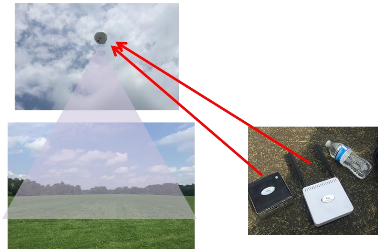
Figure 2 Deploying a standalone aerial base station.
